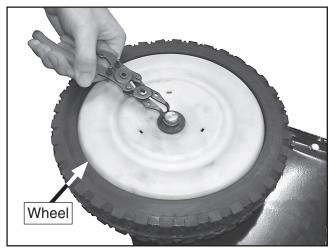
Figure 11. Retaining clip removal.
